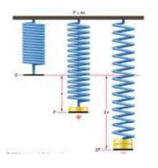
Graph showing the extension of a Spring as the weight hung from it, and hence the tension in the spring, increases.
