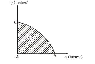
The diagram above shows a cross-section *R* of a dam. The line *AC* is the vertical face of the dam, *AB* is the horizontal base and the curve *BC* is the profile. Taking *x* and *y* to be the horizontal and vertical axes, then *A*, *B* and *C* have coordinates (0, 0),  $(3\pi^2, 0)$  and (0, 30) respectively. The area of the cross-section is to be calculated.
