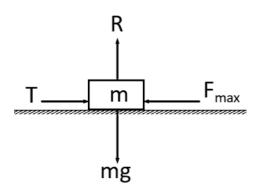
**Scenario 3**: T has reached or exceeded  $F_{\text{max}}$ , the maximum or limiting value for the friction.
