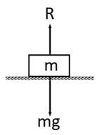
**Scenario 1:** A block is on a horizontal rough surface with no forces (other than gravity) acting on it.
