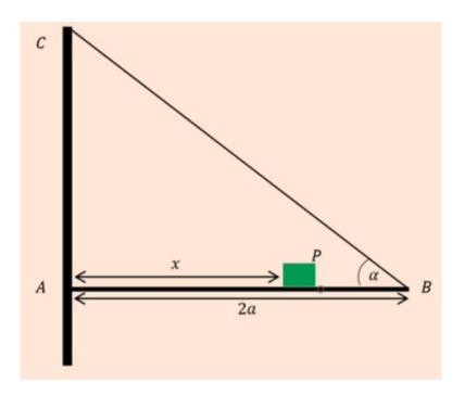
The plank is modelled as a uniform rod, the block is modelled at a particle and the rope is modelled as a light inextensible string.
